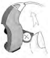
In fact, when the hearing instrument is not in use, it is recommended that you open the battery door and remove the battery. This helps to prevent excessive battery drain and allows for proper ventilation of the hearing instrument.
