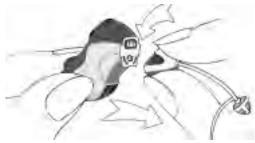
Use a damp cloth to clean the exterior of the sound tube and bud. Use the cleaning rod (provided in storage case) to clean the sound tube and bud.
